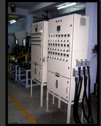
24 Zones - Hot Runner Controller for 2500 Ton Injection Molding M/C
